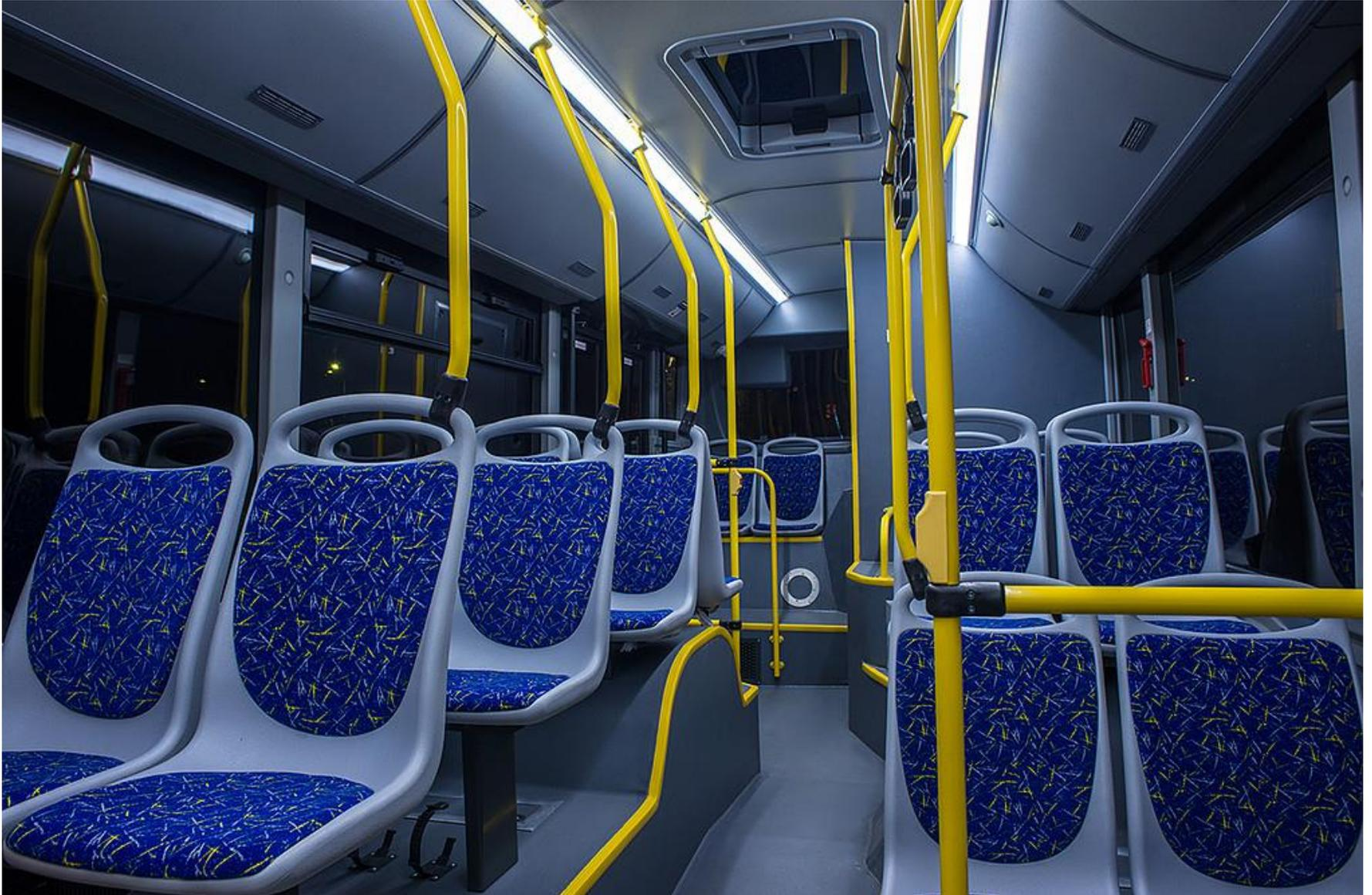
We are offering you a complete interior system for your city bus projects which is easily applicable for all kinds of sections. The air channel of the system consists of flap assemblies which are configured in different dimensions according to your needs and those flaps are also used for service/maintenance purposes as service flaps. The LED Type Light Channel is also included in our system on both sides of the ceiling.
